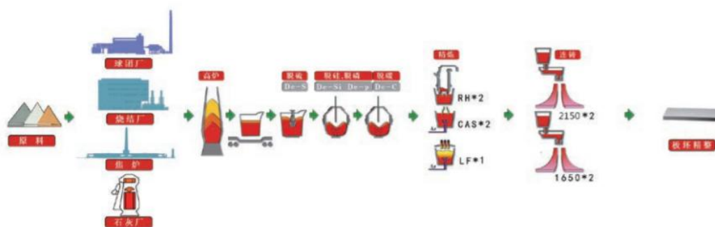
炼钢系统工艺流程图 / Flow Chart illustrating the Steel-making Process
